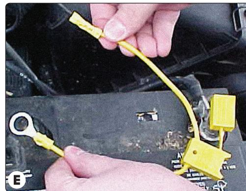
8. Reconnect the vehicle's Negative (-) battery cable and install the 15 amp fuse into the fuse holder from step 7.
