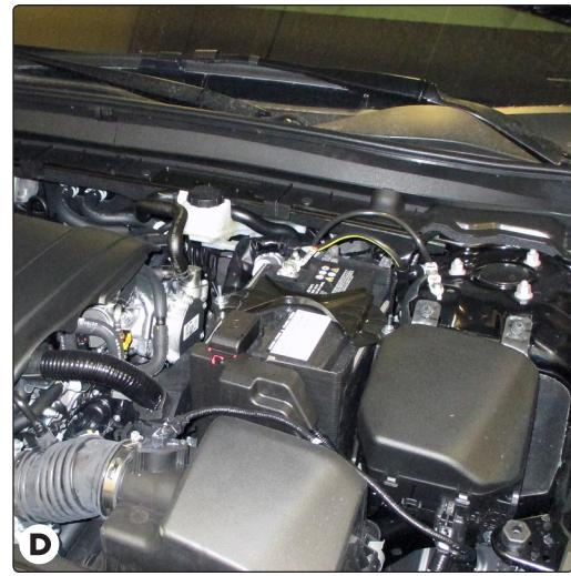
6. Route the T-One® Connector end with green wire to the passenger's side behind the panels and along the threshold.
