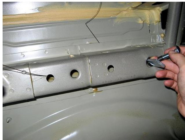
*Example of fishwire technique
