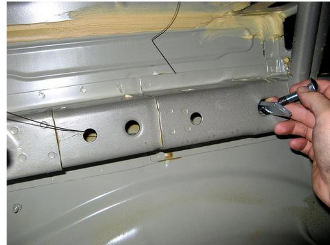
*Example of fishwire technique
