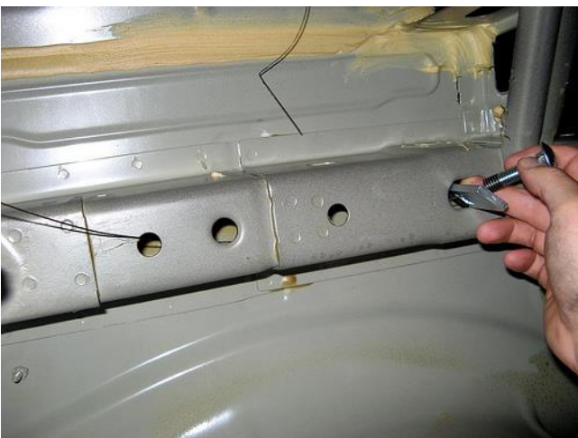
*Example of fishwire technique
