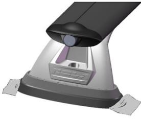
Mark mounting holes with fine tip marker or pencil
