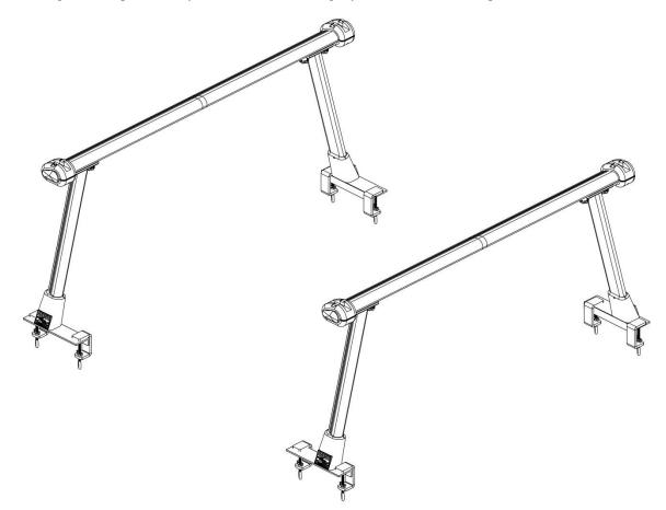
Place the previously assembled side rails into the channels of the previously installed clamps.
