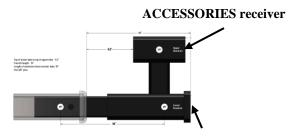
**TOWING** receiver **NOTE: Stress ring present** for towing applications
