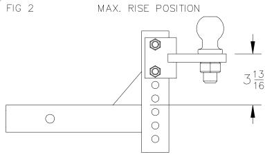
NOTE: CHECK FOR PROPER BALL MOUNT HEIGHT WITH VEHICLE & TRAILER LOADED FOR TRAVEL.
