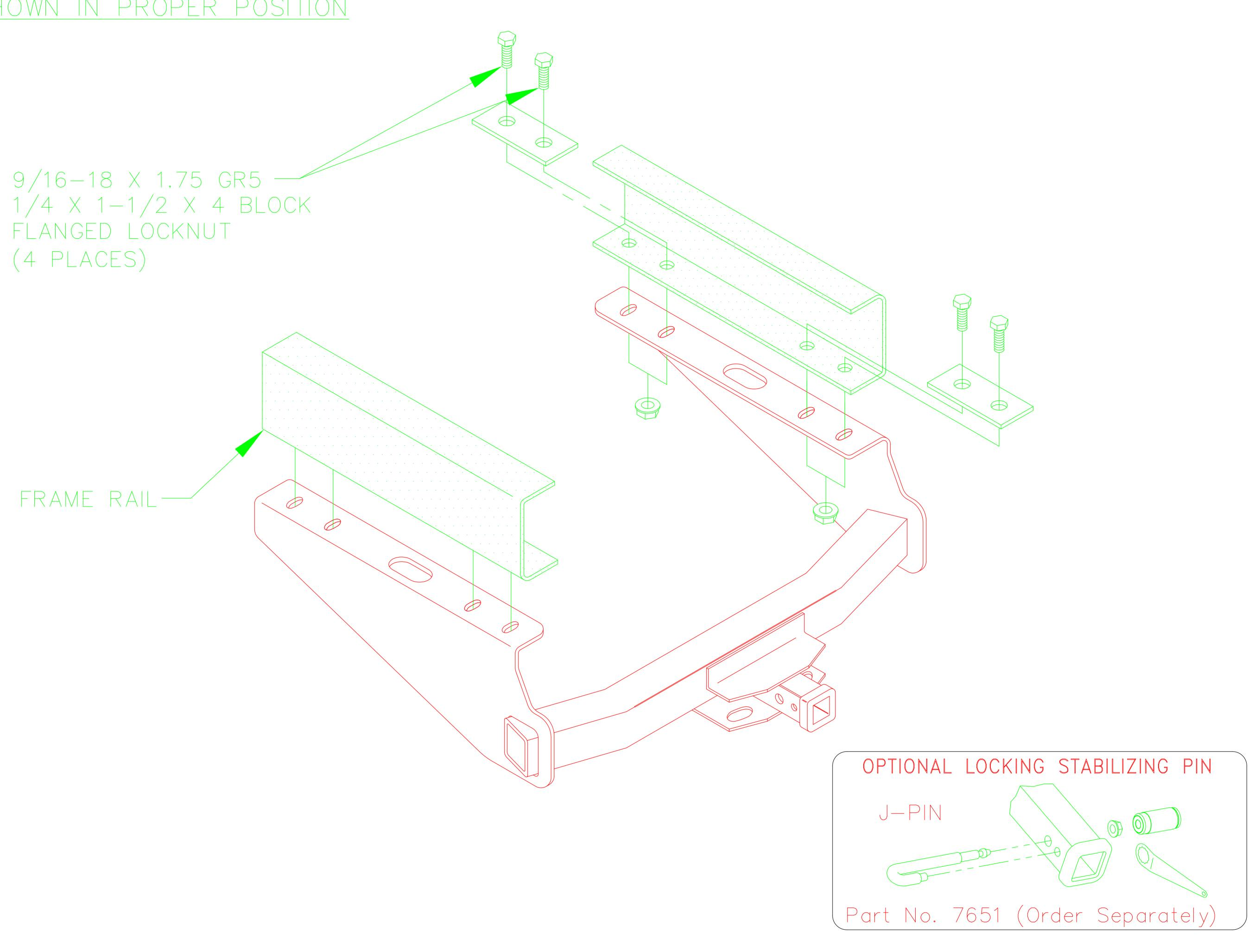
NOTE: DUE TO VEHICLE AND TIRE SIZE VARIATION SPARE TIRE MAY HAVE TO BE LOOSENED TO INSTALL HITCH.
